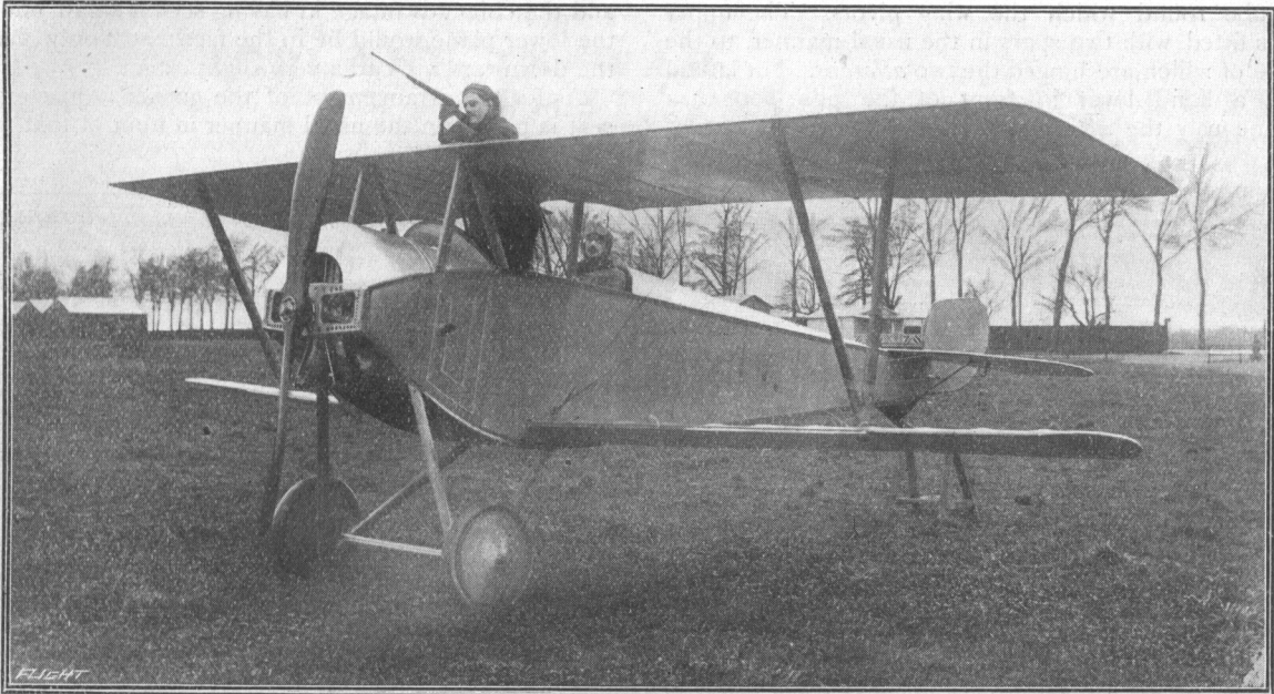
Three-quarter front view of the two-seater Nieuport biplane. The view from the pilot's seat is excellent in every direction owing to the small chord of the lower plane, whilst that of the gunner is equally good, he being able to look over the lower plane for a forward and downward view. By standing up in his seat, with his body projecting through the opening in the top plane, he is free to fire his rifle in any direction except straight downwards.
